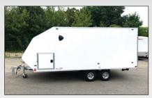
This 14-foot side-by-side model shown here has twin axles, aluminum wheels and Flo-thru yents.
