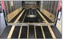
Traction mats are standard on the 7-foot wide models. Traction mats protect the floor and
