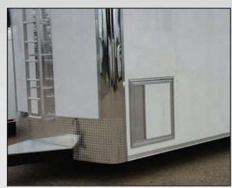
**GENERATOR DOORS -** Lockable generator doors give shelter and security for on-board power with ample ventilation.
