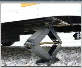
**5,000 LB SCISSOR JACKS -** Steady footing; optimal weight distribution and an extended crank handle all come with this heavy-duty accessory.
