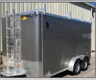
**FRONT DECK WITH LADDER -** This sturdy front deck with ladder provides easy access to roof ladder racks—safer and more convenient.
