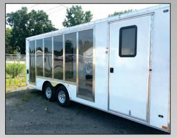
**CUSTOM SIDEWALLS -** This mobile medical trailer features clear Lexan sidewalls to allow for ambient light. Talk to your Stealth dealer about custom sidewalls.
