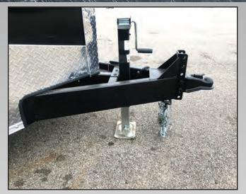
**HEAVY DUTY JACK -** This fixed-mount heavy duty jack is installed to take the maximum load on its oversized foot.
