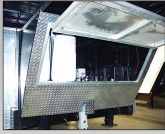
**ENCLOSED LANDING GEAR COMPARTMENT WITH ATP** - Our ATP-faced landing gear compartment with flush lock latches and baggage doors are a perfect place for tools, baggage and emergency road equipment.
