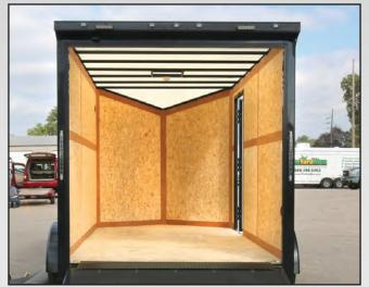
**TRANSLUCENT ROOFING-** An easy solution to light inside of the trailer during the working day—a common option for enclosed construction and landscape trailers.
