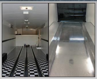
**CUSTOM FLOORING -** Choose from a variety of custom flooring materials that include checkered flag vinyl, or non-skid ATP plating (ramp-over wheel wells shown here)... and more.
