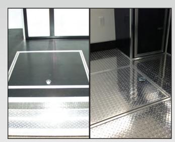
**RECESSED TIRE COMPARTMENT -** Large enough for a full-size spare trimmed to match trailer floor.
