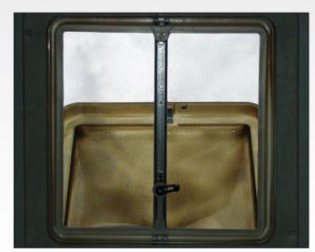
**PASSIVE ROOF VENT -** These vents can be configured to scoop or draw air into the trailer and include crank handles and screens.
