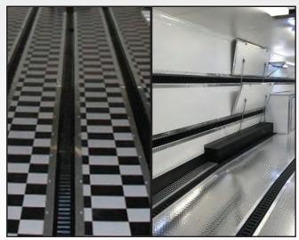
**E-TRACK WALL & FLOOR TIE DOWNS -** Flush-mount E-Track tie-downs are mounted to any point that you specify on the interior wall or floor of your trailer.
