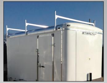
**ROOF LADDER RACK -** Welded, tubular aluminum ladder racks come in a variety of sizes to accommodate any size trailer or load.
