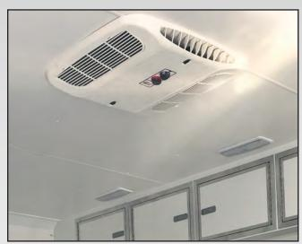
**ROOF AIR CONDITIONING -** This roof mounted airconditioning unit has directional vents, variable temperature knob, and three-position cool and fan.
